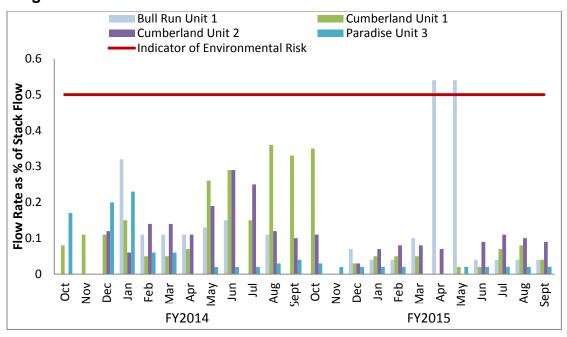
Figure 1: Flow Rates of Leaks at TVA Coal Plants<sup>10</sup> FYs 2014 and 2015
