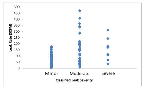
Figure 2: Leak Rates (SCFM) Versus Classified Severity
